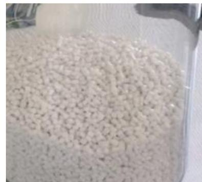
PET reclaim material obtained after transformation. It can replace virgin material for the manufacturing of various plastic based products.
